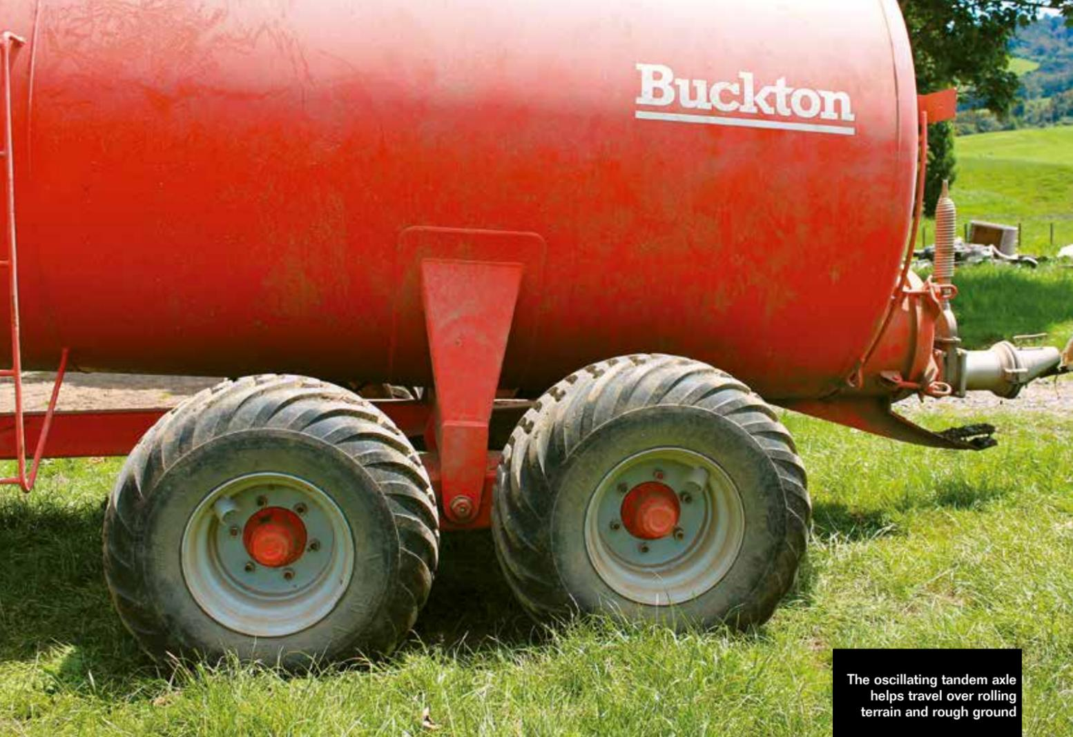
The oscillating tandem axle helps travel over rolling terrain and rough ground
