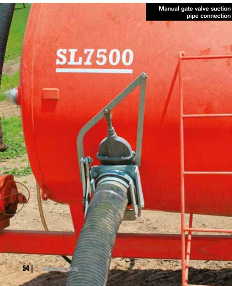
Manual gate valve suction pipe connection
