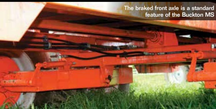
The braked front axle is a standard feature of the Buckton MS
