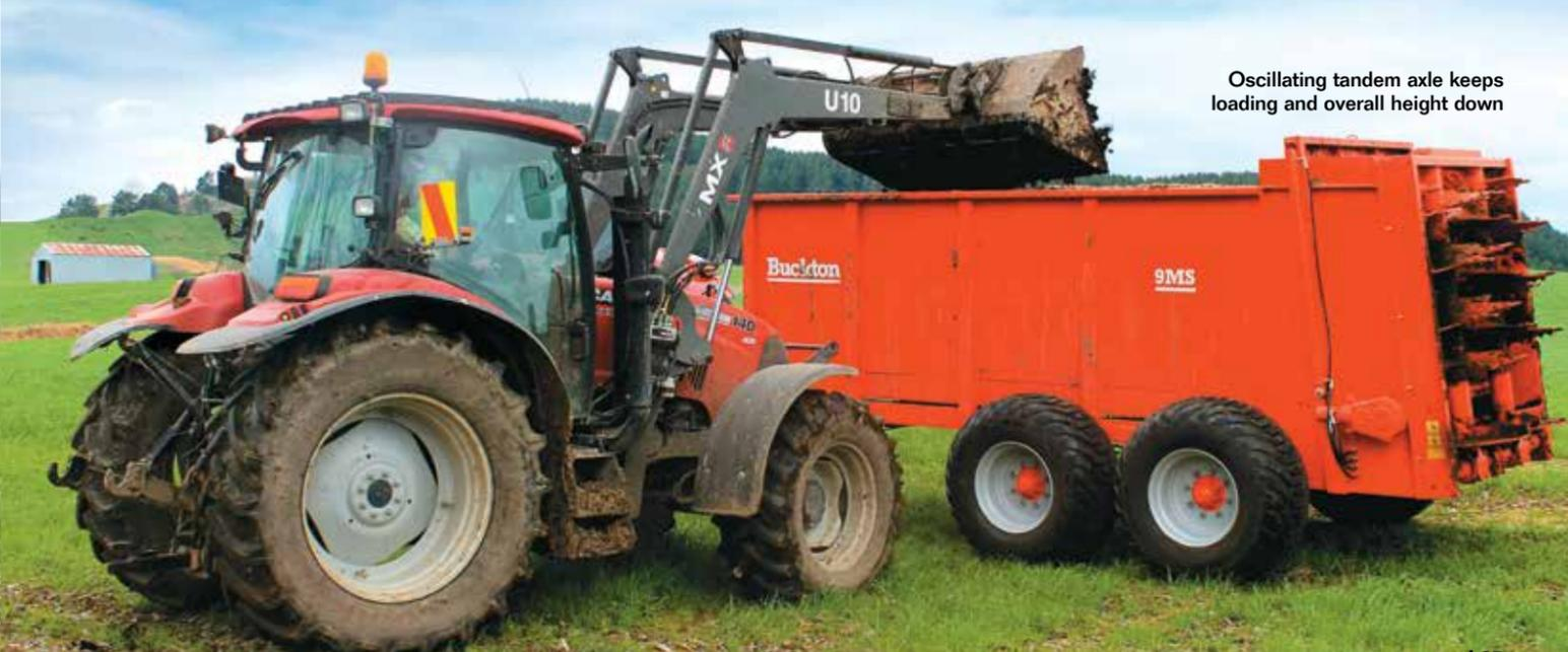
Oscillating tandem axle keeps loading and overall height down
