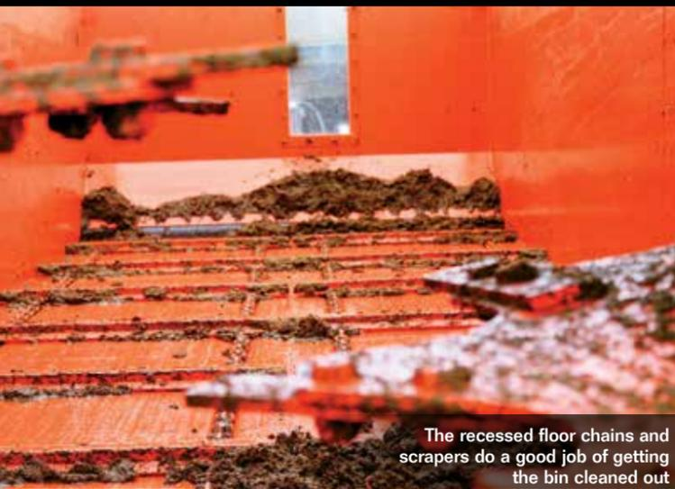
The recessed floor chains and scrapers do a good job of getting the bin cleaned out
