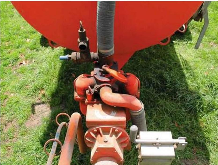
It's all pretty simple really. The PTO-driven pump has a handle on top with three positions; suck, neutral and pump. In 540 PTO speed, you can turn on the pump to start building vacuum while you connect the 150mm suction pipe (standard with 2x 4m and 1 steel probe). Once connected, filling time is four to five minutes at most.
