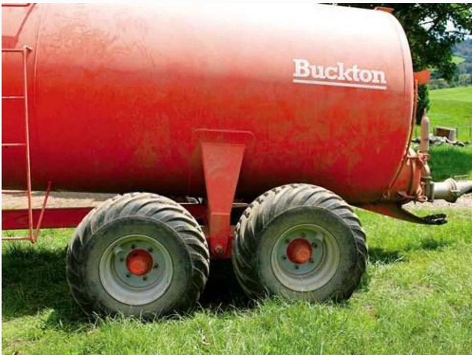
Kitted up with rear duals, the six-cylinder, 140hp machine is well-suited to the task. With no drawbar suspension, the 7500L tank still travels along nicely behind the tractor on the standard 400/60x15.5 tyres, on an oscillating axle setup. Different tyre configurations are available to suit different conditions should they be required though.
