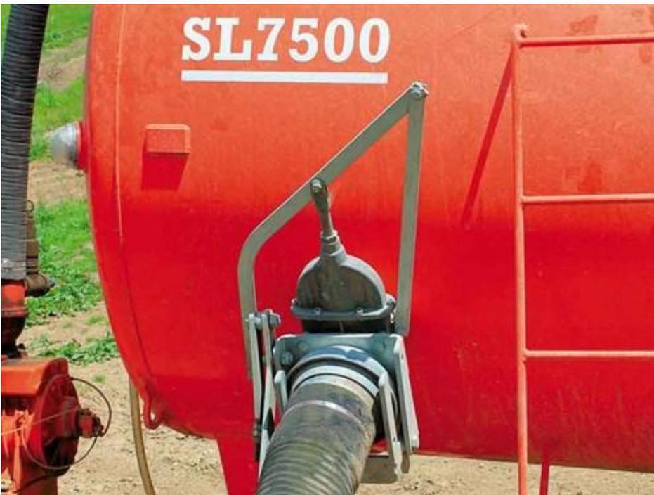
Peter said occasionally stones will get into the tank, which can cause a blockage in front of the spreader plate. Small stones in the tank sometimes don't let the rear hydraulic spreading outlet shut and seal properly, to create a vacuum for filling next time. Both issues are easily fixed though. The top hatch and rear opening allow access to hose out the tank if you have sucked in stones.
