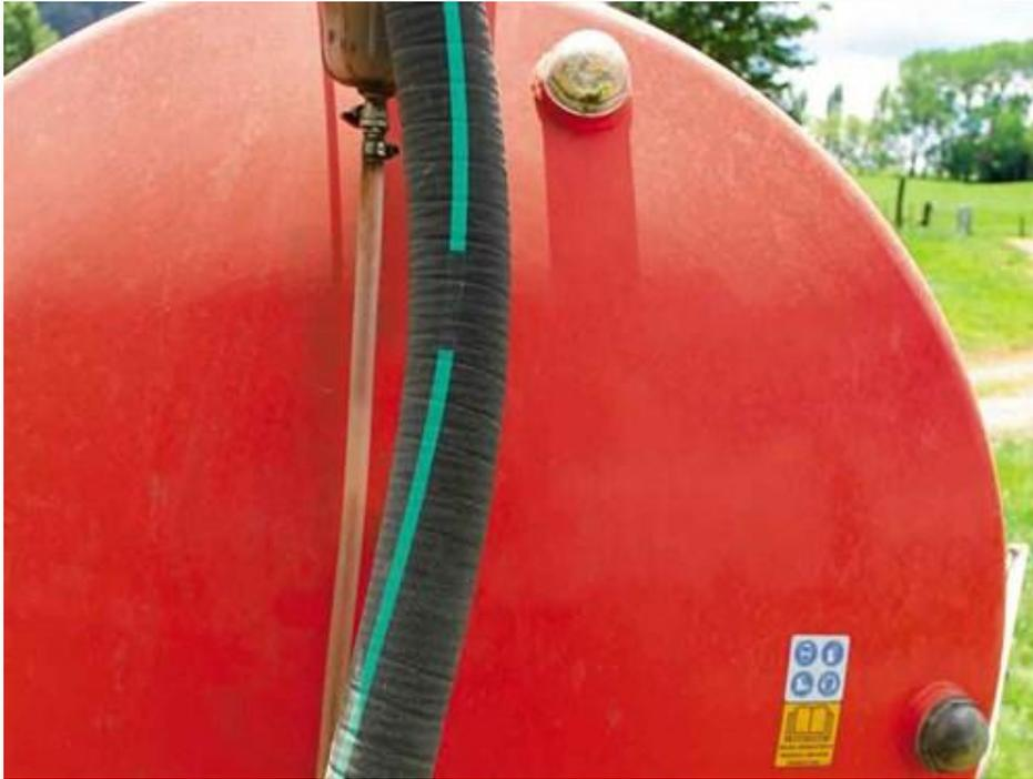
Once full, you are ready to spread when you get to your paddock. The 7500L Buckton tanker is fitted with an 8000L/min pump as standard, which seemed to be a good size for this tank.
