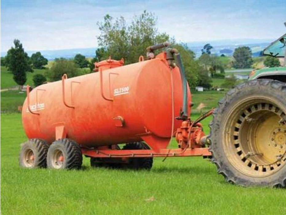
The only hydraulic connection required is for the rear outlet to begin spreading. When you want to stop spreading, just shut the rear outlet again. The basic rear spreader plate is just that; it does the job perfectly well for a fraction of the cost of a dribble bar or injector system.
